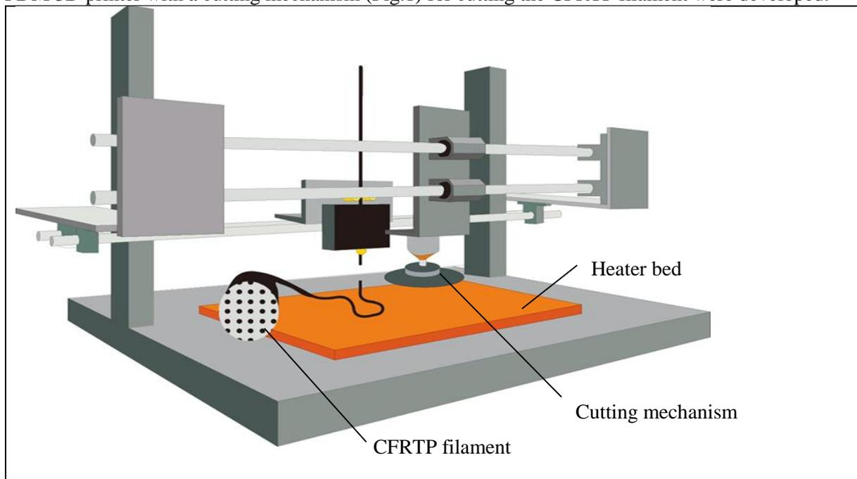
**Figure 1:** Schematic diagram of the 3Dprinter with continuous carbon fiber and cutting mechanism.
